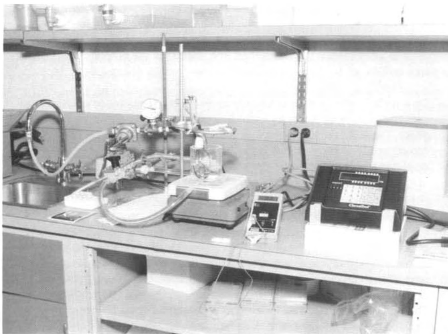
Washing machine thermal cycler built by leadership teachers successfully amplified human DNA polymorphisms.
